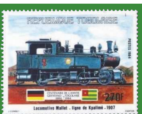
ABOVE: 270f design showing a locomotive used on the Lomé-Kpalimé railway, the second in Togo. Completed in 1907, it ran inland for a distance of about 75 miles, and its most important cargo was cocoa beans. The Mallet-type engine was an articulated loco with an adjustable wheelbase
